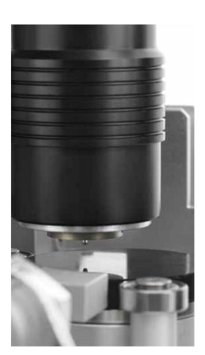
Shore A hardness measurements are based on the precise application of force and the subsequent measurement of probe displacement.
