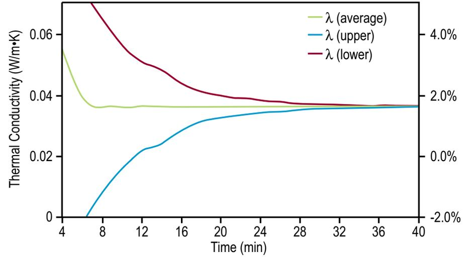
**Calibrations for lateral heat loss and interface resistance.** Gives users the ability to test thick samples, and materials of higher thermal conductivity.
