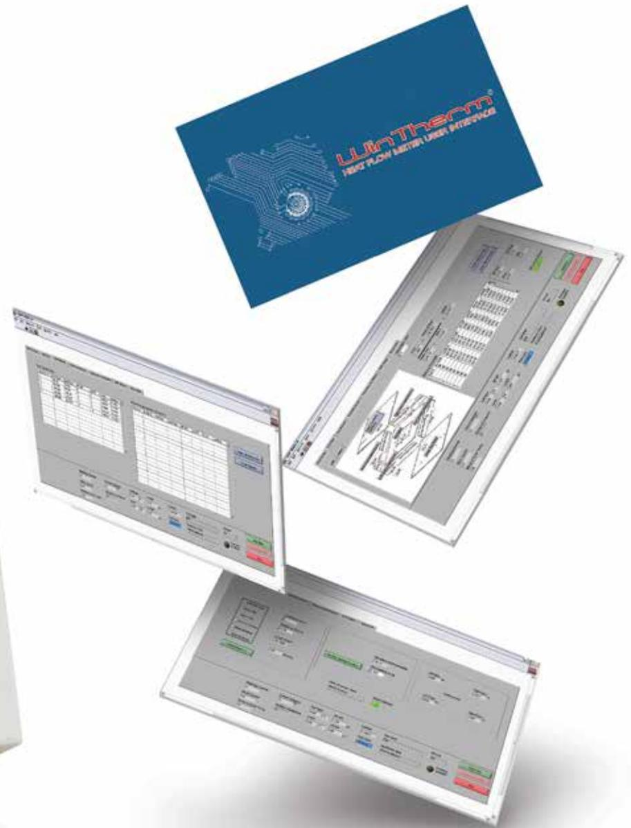
**Accelerated testing** - the average heat flow of the upper and lower heat flux sensors is calculated, and stabilizes much faster than individual signals. Accurate measurements (to within +/- 0.4%) can be made in less than half the time, increasing laboratory throughput.
